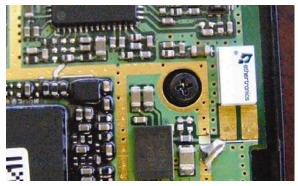
Ethertronics' Savvi series of Isolated Magnetic Dipole<sup>TM</sup>(IMD) antennas deliver on the key needs of device designers for higher functionality and performance in smaller/thinner designs. These innovative antennas provide compelling advantages for Bluetooth<sup>®</sup> enabled cell phones, media players and other mobile devices.
