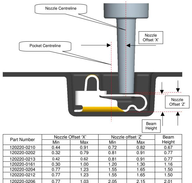
These recommendations should be used to set up the SMT pick and place offsets. The offsets will require fine tuning for each machine type and speed of operation in order to gain maximum pick and place performance.
