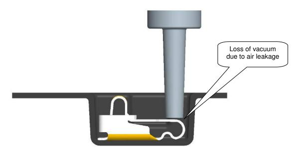
If minimum offset in 'X' is exceeded, there could be damage to the contact pre-load tag features
