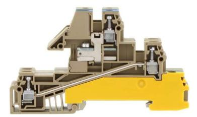
Three-wire installation terminal, Screw connection, Mounting type: Mounting rail TS 35/7.5, Rated cross-section: 2.5 mm<sup>2</sup>, Width: 12 mm, Colour: Beige
