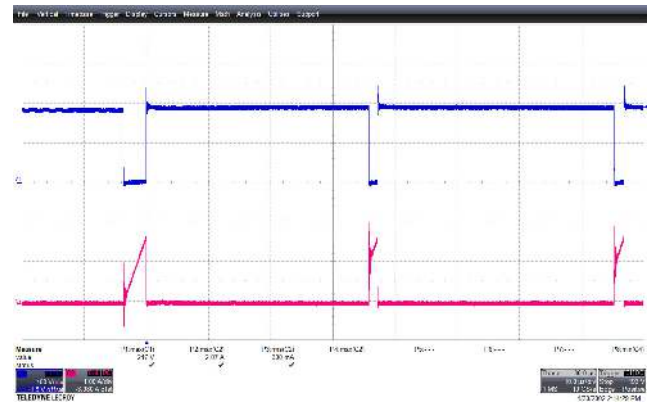
Figure 103 – 132 VAC 60 Hz, Short-Start-up. Zoom in CH1(Blue): V_D , 100 V / div., 10 \mu s / div. CH2(Pink): I_D , 1 A / div.
