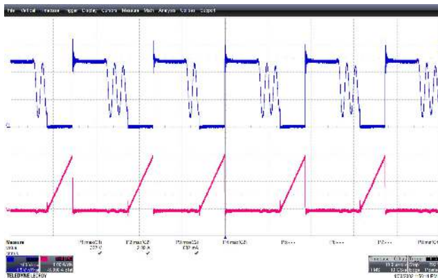
Figure 62 – 100 VAC 60 Hz, 20 V Full Load Normal. CH1(Blue): V_{DS} , 100 V / div., 20 ms / div. CH2(Pink): I_{DS} , 1 A / div. V_{DS} = 322\text{ V} , I_{DS} = 2.09\text{ A} .
