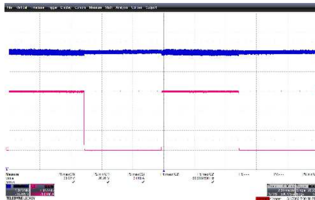
Figure 81 – 132 VAC 60 Hz, 0-3 A Transient Load. CH1(Blue): V_{OUT} , 1 V / div., 2 ms / div. CH2(Pink): I_{OUT} , 1 A / div. V_{OUT(MAX)} = 20.62\text{V} , V_{OMIN} = 20.26\text{ V} .
