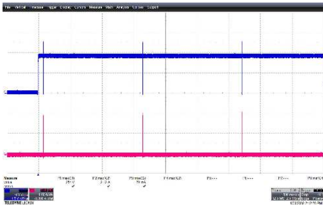
Figure 102 – 132 VAC 60 Hz, Short-Start-up CH1(Blue): V_D , 100 V / div., 1 s / div. CH2(Pink): I_D , 1 A / div.
