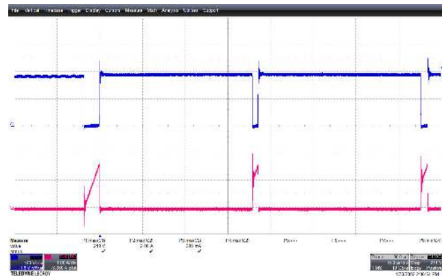
Figure 99 – 132 VAC 60 Hz, Output Short Normal. Zoom in CH1(Blue): V_D , 100 V / div., 10 us / div. CH2(Pink): I_D , 1 A / div.
