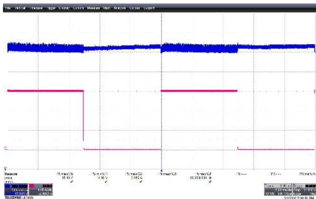
Figure 82 – 100 VAC 60 Hz, 0-3 A Transient Load. CH1(Blue): V_{OUT} , 1 V / div., 2 ms / div. CH2(Pink): I_{OUT} , 500 mA / div. V_{OUT(MAX)} = 15.19\text{ V} , V_{OMIN} = 14.9\text{ V} .
