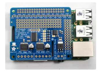
Place the HAT on top so that the short pins of the 2x20 header line up with the pads on the HAT
