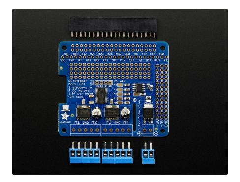
Comes with an assembled & tested HAT, terminal blocks, and 2x20 plain header. Some soldering is required to assemble the headers on. Stacking header not included, but we sell them in the shop so if you want to stack HATs, please pick one up at the same time. (http://adafru.it/2223)
