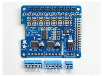
Now grab the 3.5mm-spaced terminal blocks. These will let you quickly connect up your motor and power supply using only a screw driver
