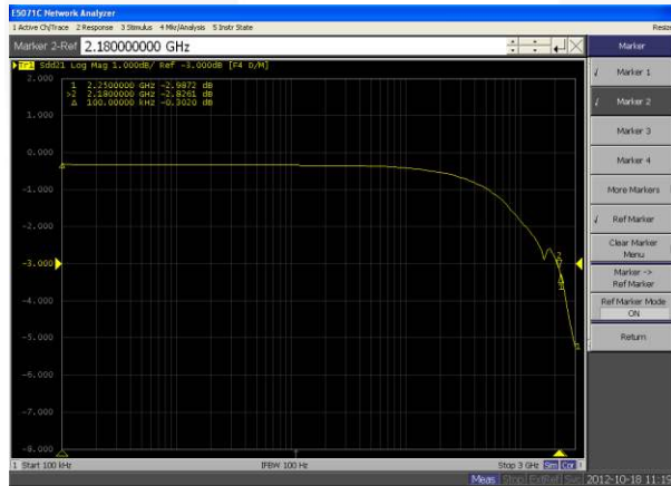
Figure 17. USB Path SDD21 Insertion Loss Curve
