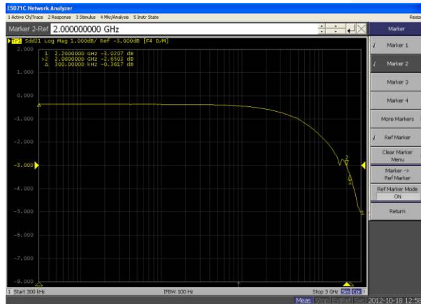
Figure 16. MHL Path SDD21 Insertion Loss Curve
