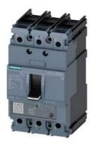
circuit breaker 3VA5 UL frame 125 breaking capacity class H 65kA @ 480 V 3-pole, line protection TM230, FTAM, In=90A overload protection Ir=90A fixed short-circuit protection Ii=5...10 x In UL489 SB (naval), 50 deg. cel. nut keeper kit on both sides
