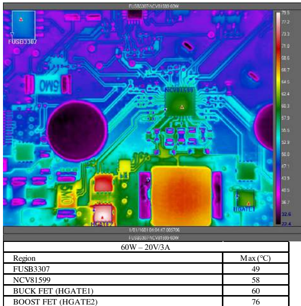
Figure 54 - Thermal image and data for 60W (20V/3A)
