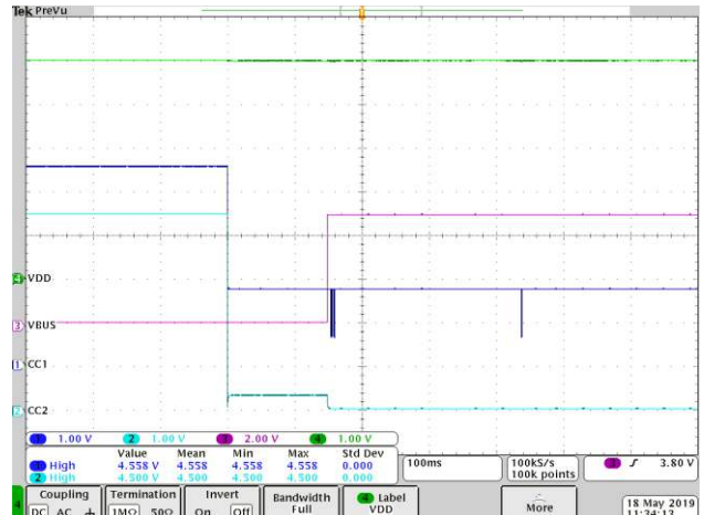
Figure 47 - VCONN when cable marker cable is attached (FUSB3307 w/3A support)
