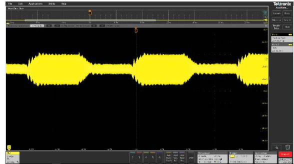
Figure 21 - Transient load on 15V VBUS
