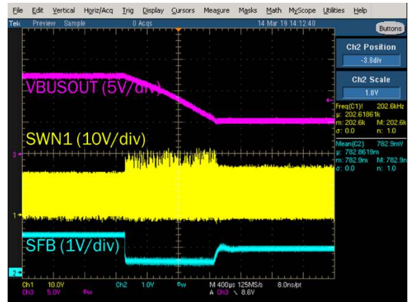
Figure 11 - 12V to 5V transition with no load
