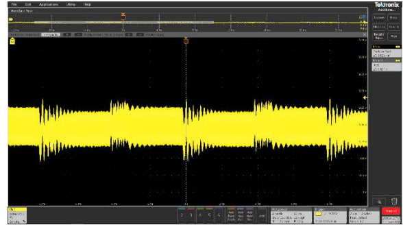
Figure 19 - Transient load on 9V VBUS
