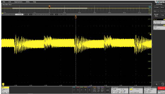
Figure 18 - Transient load on 5V VBUS
