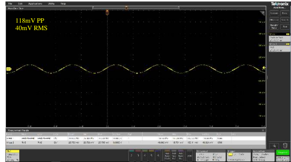
Figure 30 - VBUSOUT ripple for 15V/0A
