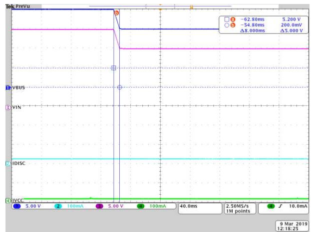
Figure 36 - VBUS discharge, from 20V to 15V, with a 500mA load
