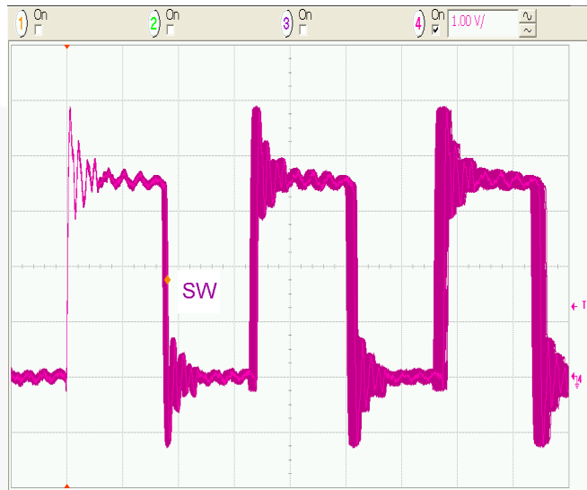
Figure 39. SW-Node Jitter (Infinite Persistence), I_{LOAD} = 200mA , 50ns/div .
