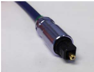
Figure 55. TOSLINK Connector and Optical Fiber Cable for S/PDIF Input and Output
