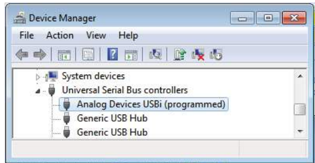
Figure 10. Confirming Successful Driver Installation Using the Device Manager
