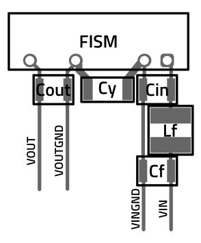
The layout above has been evaluated to provide the optimal performance in terms of transient response, efficiency, ripple and EMI. The design footprint can be reduced at the expense of performance in these parameters. The following recommendation should be followed when designing the layout:
