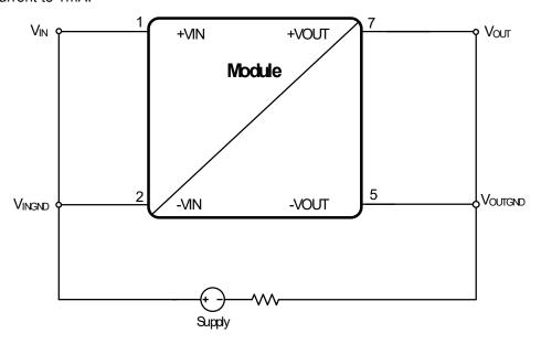
Parameters Supply Device: Current limit set 1mA, test voltage 3000 VDC, test time 60s.
