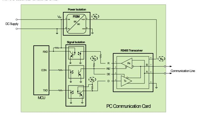
To set up an isolated communication, different functional units are required. The data for the RS485 transceiver is provided by the Micro Controller Unit (MCU), which in turn receives data from the RS485 transceiver. With the use of optocouplers the signal isolation unit can achieve galvanic isolation of the signals. A power isolation unit - a DC/DC converter power module - attains galvanic isolation of the grounds between the signal isolation unit and the transceiver unit.
