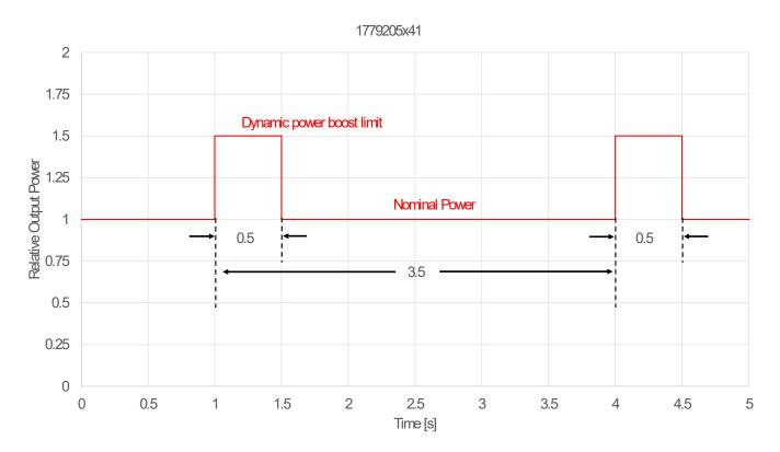
**Note:** The overload current of 150% of  $I_{OUT}$  can be supplied for maximum 0.5s and requires a 3s recovery time till next overload event.
