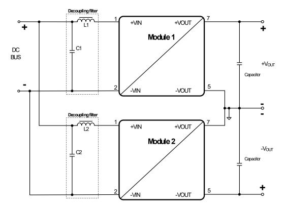
For using long supply lines or different line length for each 1779205x11 it is recommended to decouple each power module with an additional LC- filter. The decoupling LC-filter is also recommended if the supplying dc bus has a high impedance so that high voltage swings at the input of each power module could be present. As initial values, the EMI filter shown for every part number can be used. See also "Primary side parallel connection".
