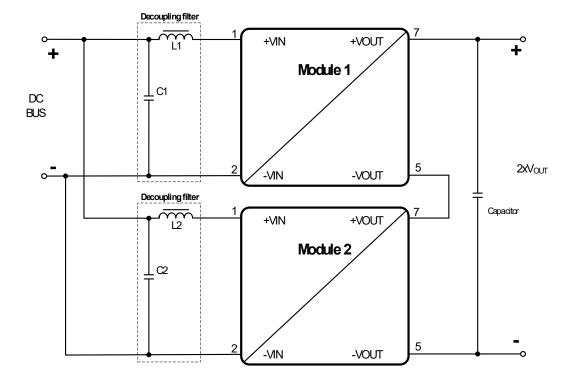
In case of using long supply lines or different line length for each 1779205x11 it is recommended to decouple each power module with an additional LC filter. The decoupling LC filter is also recommended if the supplying dc bus has a high impedance so that high voltage swings at the input of each power module could be present. As initial values, the EMI filter shown for every part number can be used. See also "Primary side parallel connection".
