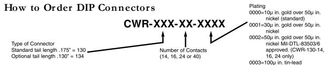
EXAMPLE: CWR-130-16-0002 is part number for a 16-pin DIP connector with .175 in. tails and 50µ in. gold over 50µ in. nickel contacts
