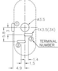
Recommended PCB Layout Top View
