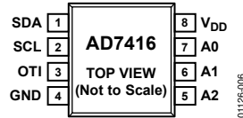
Figure 7. AD7416 Pin Configuration (SOIC/MSOP)
