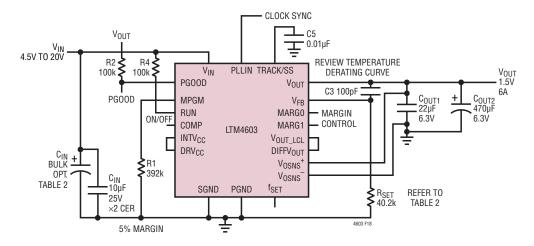
Figure 18. Typical 4.5V to <sub>20VIN</sub>, 1.5V at 6A Design
