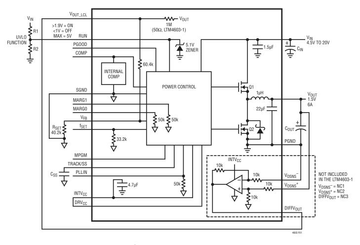
Figure 1. Simplified LTM4603/LTM4603-1 Block Diagram
