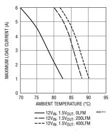
Figure 11. No Heat Sink 12V<sub>IN</sub>
