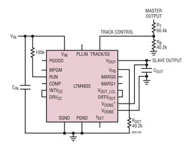
Figure 5. Coincident Tracking Schematic
