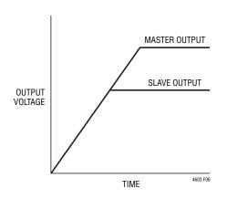
Figure 6. Coincident Output Tracking Characteristics
