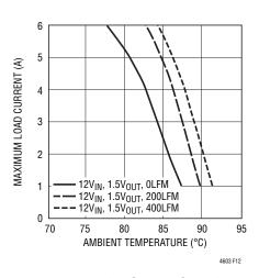
Figure 12. BGA Heat Sink 12V<sub>IN</sub>
