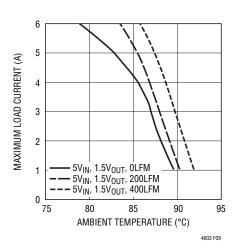
Figure 9. No Heat Sink  $5V_{IN}$
