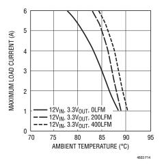
Figure 14. 12V<sub>IN</sub>, 3.3V<sub>OUT</sub> BGA Heat Sink
