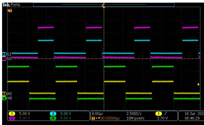
Figure 2. Example Input and Output Waveforms (Green and Magenta are PWM Inputs, Yellow and Blue are Driver Outputs)
