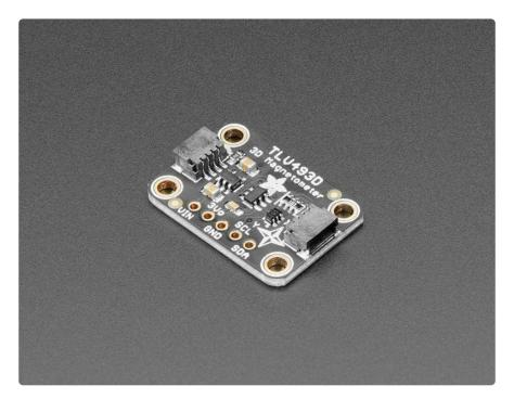
We've also outfitted the breakout with <u>SparkFun Qwiic</u> () compatible <u>STEMMA QT</u> () connectors to allow you to use it with other similarly equipped boards without needing to solder. Because the TLV394D "speaks" I2C, you only need two wires (in addition to power) to interface with your microcontroller, and you can share those pins
