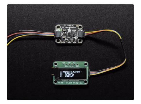
The TLV493D 3-axis magnetometer is a great little sensor for detecting magnets in 3D. () In fact, the manufacturer Infineon suggests it could be used to make a joystick! You could also use it for other cool things like detecting objects with magnets attached, like the lid of a box, or maybe a statue that unlocks your secret lair when placed on your mantle?
