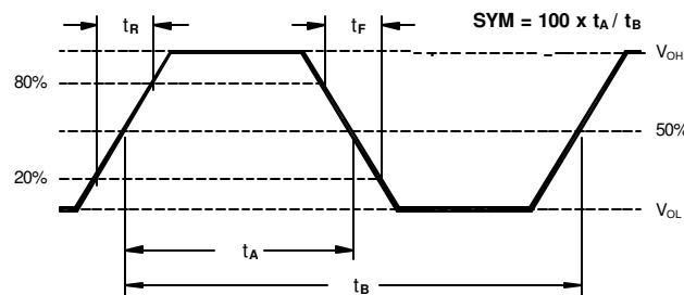
Figure 2. PECL Waveform
