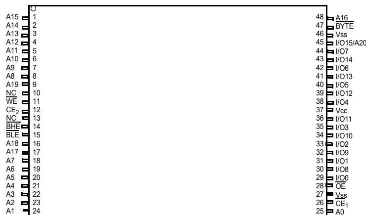
Figure 2. 48-pin TSOP I pinout (Top View) [2, 3]
