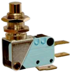
Telescopic plunger and adjustable fixing . 4mm overtravel. Metal version for heavy duty (SP9603)
