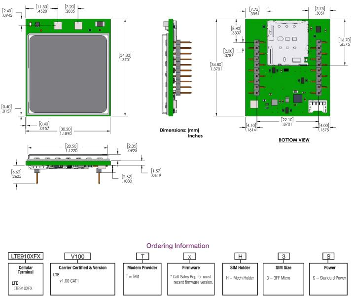
Example: Part Number – LTE910XFXV100TAH3S = LTE Cellular XF Embedded Modem; Telit Modem; Current Firmware; Mech SIM Holder; SIM Card Size 3FF; Standard Power
