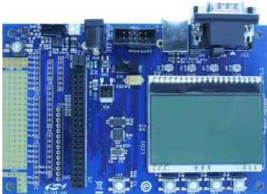
Figure 1. MSC-DBSB8 Software Development Board (SDB)
