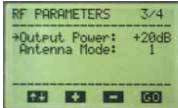
Figure 18. Screen 3: RF Parameters (Antenna Diversity Card Fitted)
