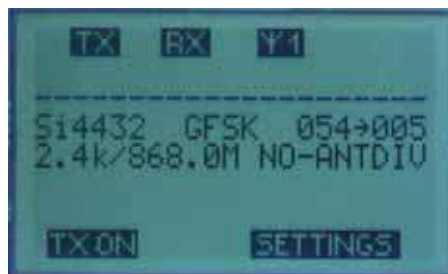
Figure 21. Non-Antenna Diversity Testcard
