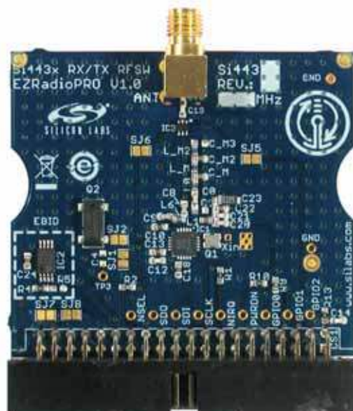
Figure 17. Single-Ended TX and RX Testcard
