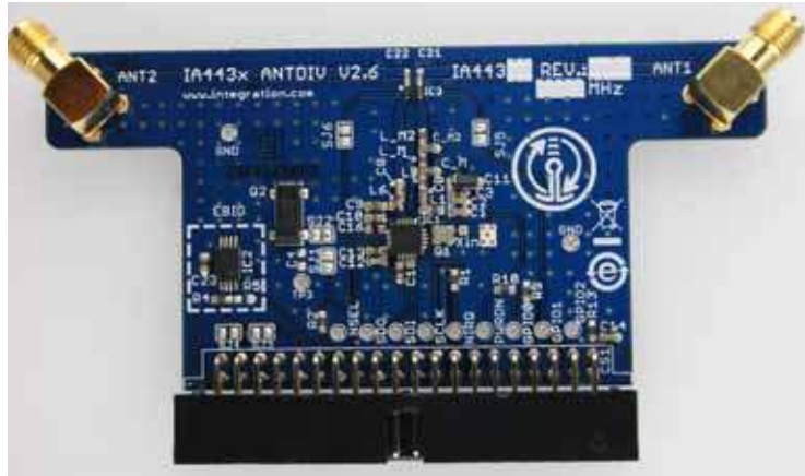
Figure 15. Antenna Diversity Testcard (May be Ordered Separately)
