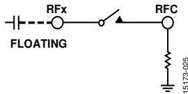
Figure 56. Series Capacitor Directly Connected to MEMS Switch
