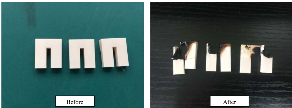
Figure 3 – visual check for GWT 750°C test
