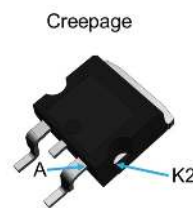
Figure 12. Creepage without top coating
