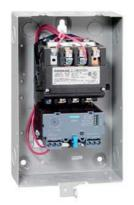
Non-reversing motor starter Size 1 3/4 Three phase full voltage Solid-state overload relay OLRelay amp range 10-40a 240VAC 50HZ / 277VAC 60HZ coil Combination type Indoor general purpose use
