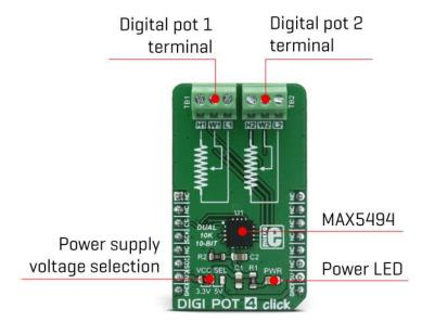
All the communication with the control logic of the MAX5494 is done through the SPI, so all the SPI signals are routed to the appropriate mikroBUS<sup>™</sup> pins. The CS pin is held high, preventing the SPI communication, so as always - to initialize the SPI communication, the CS pin needs to be pulled LOW by the MCU.
