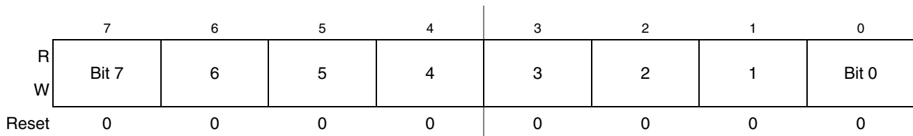
Figure 16-11. TPM Counter Modulo Register Low (TPMxMODL)
