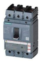
circuit breaker 3VA5 UL frame 250 breaking capacity class C 100kA @ 480 V 3-pole, line protection TM230, FTAM, In=90A overload protection Ir=90A fixed short-circuit protection li=5...10 x In nut keeper kit on both sides
