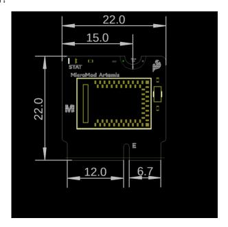
Each processor board follows the M.2 standard of '2222' or 22x22mm overall size.
