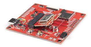
The Processor Board will stick up at an angle (at around 20°), as seen here:
