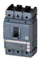
circuit breaker 3VA5 UL frame 250 breaking capacity class H 65kA @ 480 V 3-pole, line protection TM210, FTFM, In=100A overload protection Ir=100A fixed short-circuit protection Ii=10 x In UL489 SB (naval), 50 deg. cel. nut keeper kit on both sides
