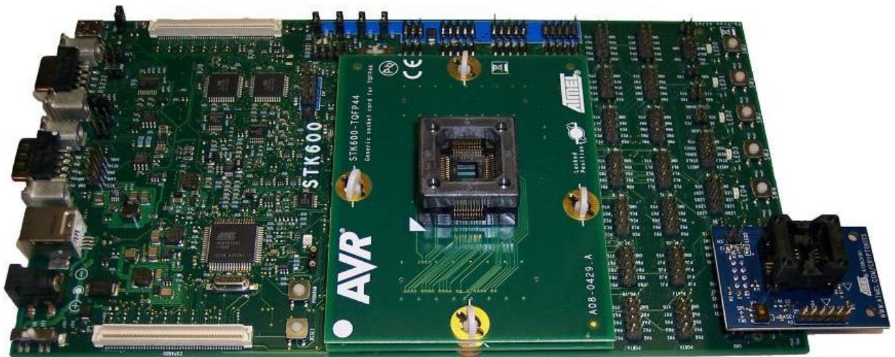
Figure 2-2. Atmel AT88CK101BK8 adapter board mounted to STK600
