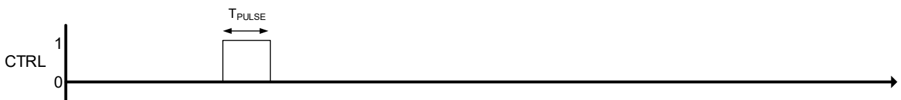
Figure 7.2: Master Output signal on CTRL to force a Reseed Condition.
