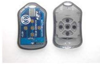
Figure 1. Si4010 Universal Key Fob Board and Plastic Case (P/N 4010-KFOB-434 and MSC-PLPB_1)
