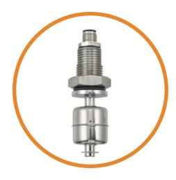
The SSF25 series is a compact vertical internally mounted device. Mounting is in the top or bottom of the tank from the inside, so requires access to the inside of the tank.
