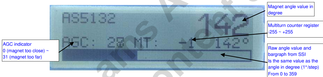
Figure 2: LCD display in standalone mode (9V battery or USB powered without GUI)
