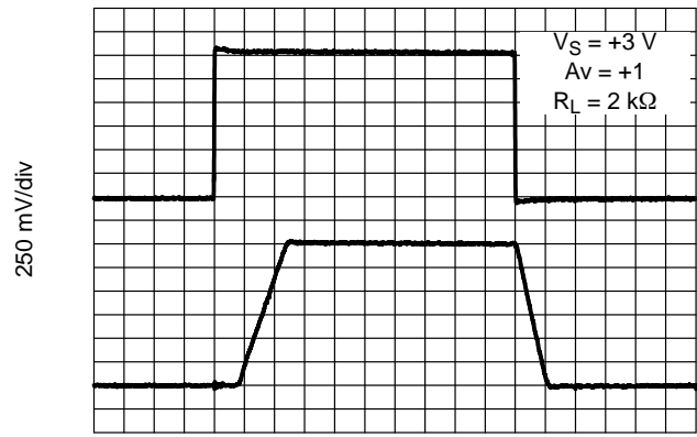
Figure 24. 3 V Non-Inverting Large Signal Pulse Response
