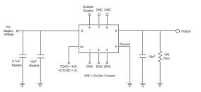
TV Series Clipped Sinewave Test Circuit
