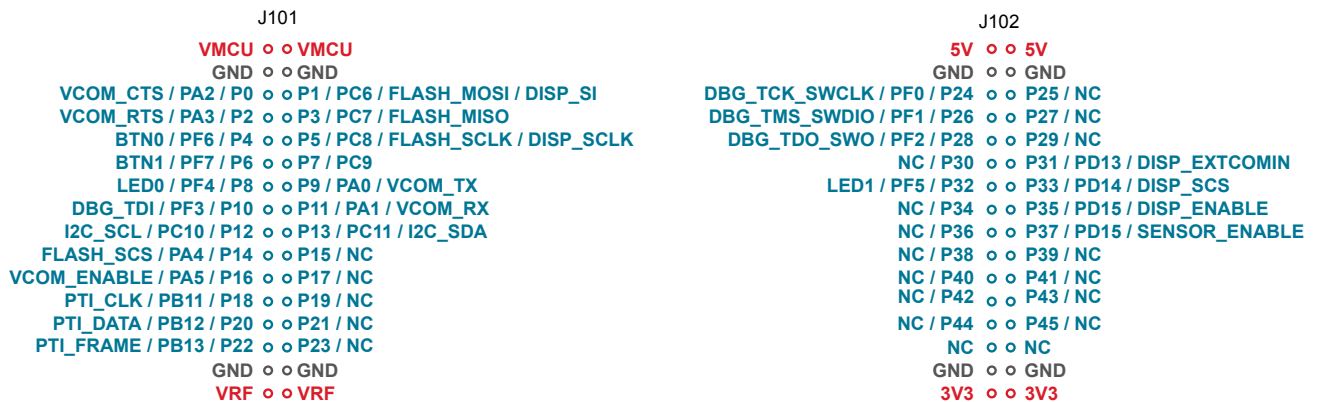
Figure 4.2. Radio Board Pin Mapping on Breakout Pads
