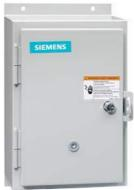
Non-reversing motor starter, Size 0, Three phase full voltage, Solid-state overload relay, OLRelay amp range 0.25-1a, 550/575 600 50/60HZ coil, Non-combination type, Enclosure type 12, Dust/drip proof for indoors, Extra-wide enclosure
