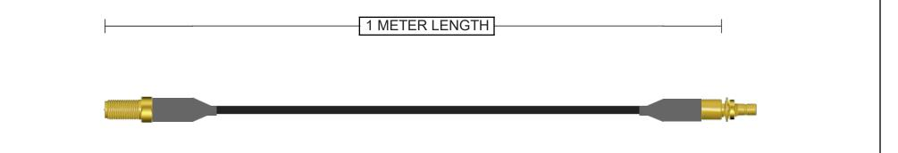
Connector A 132116RP SMA Jack Straight Brass Gold + Heatshrink 50 Ohm RG-58 Continuity/Hi-Pot Connector B 142331 SMB Jack Straight Bulkhead - Rear Mount Brass Gold + Heatshrink
