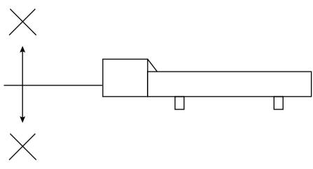
3. When the board warps greatly due to solder flow, the socket may rise up from the board.Please limit as much as possible this board warpage due to solder flow.
