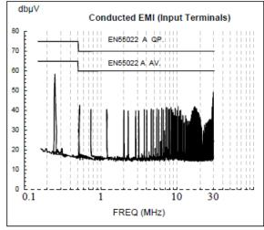
To meet class B for the above standards, it is necessary to fit a 3.3 μF ceramic capacitor across the input terminals.
