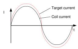
Coil current does not have optimum shape
