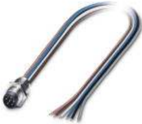
Sensor/actuator flush-type plug, 6-pos., M8, front/screw mounting with M8 fastening thread, with 0.5 m TPE litz wire, 6 x 0.14 mm 2
