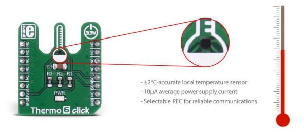
One shot reading allows for the lowest power consumption - down to 5uA, if there is no demand for continuous temperature conversion. The device remains in standby state, as long as there is no read command. Read command (writing 1 to the bit 0 of the config register) will wake up the device and read the temperature data immediately, after which it will revert to standby mode again. This allows for a very low average power consumption.
