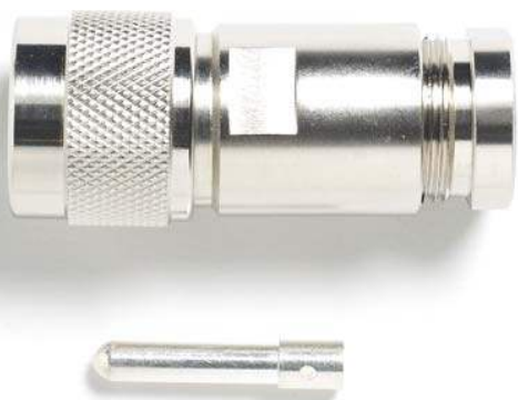
Model 73059 UHF Plug, Clamp Type, RG8, 9, 11, 63, 87A, 213, 214, 225
