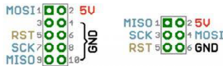
AVR ISP pinouts – top view.
