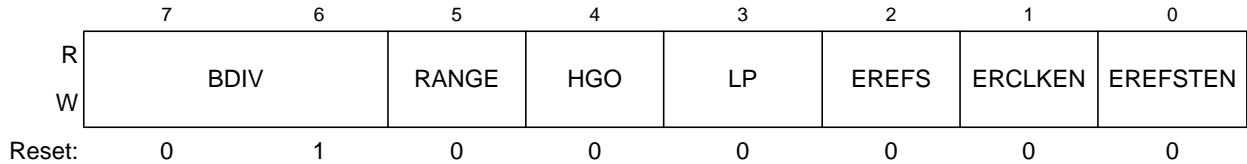
Figure 11-4. ICS Control Register 2 (ICSC2)
