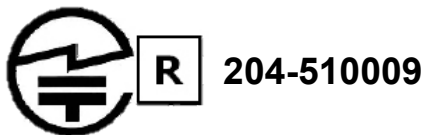
Figure 7: Giteki mark, and the ODIN-W260/ODIN-W262 MIC certification number. The “Indoor use only” information translated into Japanese below is mandatory if the product is operating in the 5.2/5.3 GHz band.
